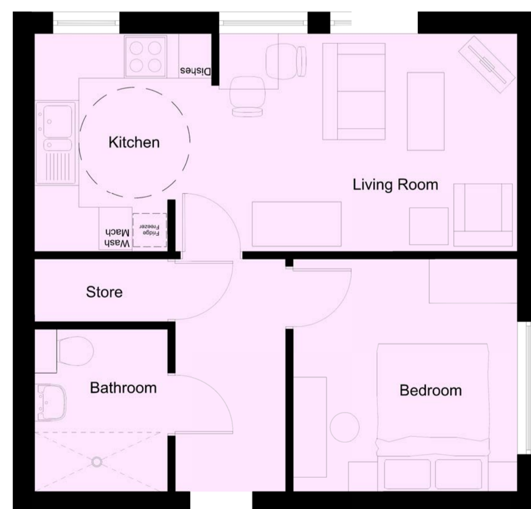
Typical Refurbished Small 1 Bedroom Flat Area - 40.5 sq m
